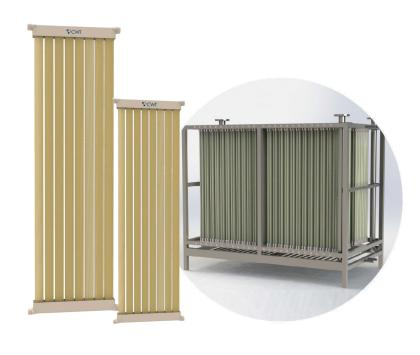
Fiber enhanced MBR membrane components from CWT's have following advantages. The hollow fiber membrane has higher mechanical properties, better pressure resistance, and higher permeability through porous structure. Moreover, the membranes have better anti-pollution and hydrophilic properties, and better separation efficiency.
